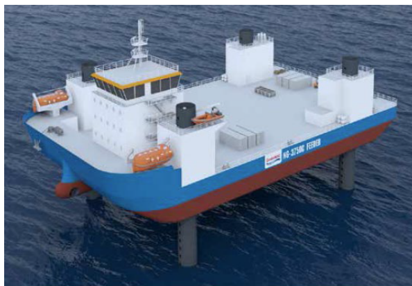
FIGURE 10.3-2: EXAMPLE OF A FEEDER BARGE (GUSTOMSC NG-3750C-FEEDER)
